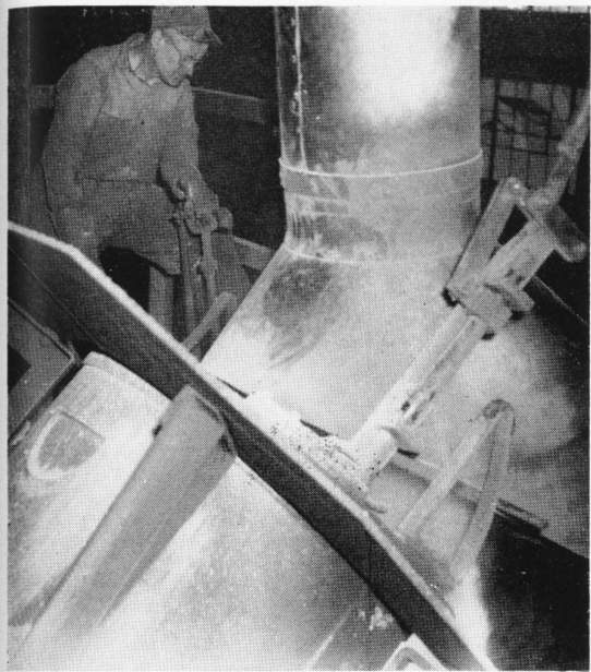
Emile Despins, lineman in the Casting Shop, opens a compressed air valve to tilt an Ajax furnace so it will pour its molten charge.
