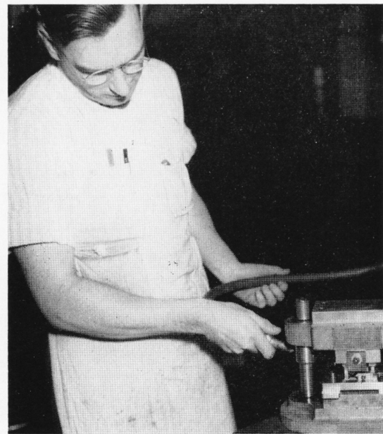
Edward Stuart in Tool Room 1 cleans a tool with the handy nearby airline. It's an ideal way to get dust and chips out of busy tools.
