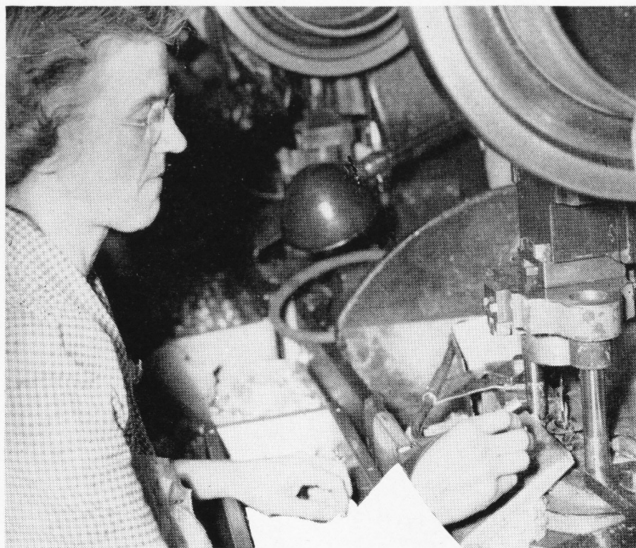
Thousands of machines in all parts of Scovill use compressed air to quickly eject work from tools and dies. Here's Caroline Lovely operating such a machine in Press 2. Having air lines to help greatly speeds up production and makes the operation safe.
